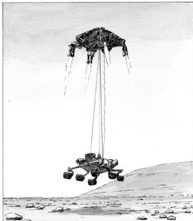
The *Curiosity* rover is on Mars, studying the Martian climate and geology and looking for substances associated with life. *Curiosity* is the size of a small car. It is so big and heavy—about five times larger than earlier rovers—that it couldn't use an airbag-landing system. Instead, it used a rocket-propelled sky-crane that lowered it gently to the surface.
